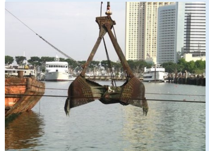
Environmental bucket (above) Clamshell bucket (below)
